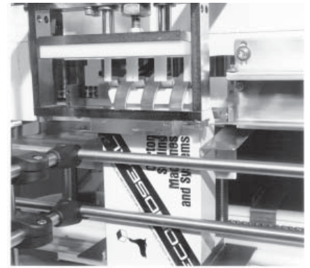
Top of carton is closed - either tuck (as shown) or glue method.
